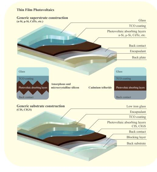
NSG TEC<sup>™</sup> Sodium Block is used for CIS/CIGS applications. It includes a sodium barrier layer, which offers manufacturers improved product stability and increased process throughput.
