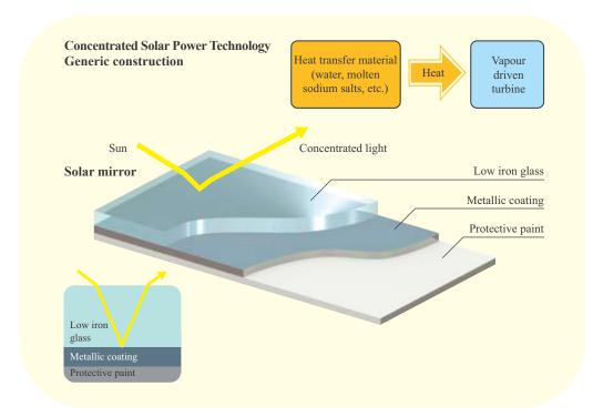
Since the sunlight has to travel through the glass twice before reaching the heat transfer material, very high light transmittance, low absorptance glass such as Pilkington **Optiwhite<sup>™</sup>** S or Pilkington **Microwhite<sup>™</sup>** is required for this application.
