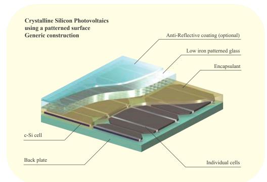
The glass type normally used for this technology is low iron rolled glass such as Pilkington **Sunplus<sup>TM</sup>**, often in toughened form, combined with an Anti-Reflective (AR) coating, to ensure that the maximum solar radiation reaches the PV cells. It is also possible to use low iron float glass such as Pilkington **Optiwhite<sup>TM</sup>**.
